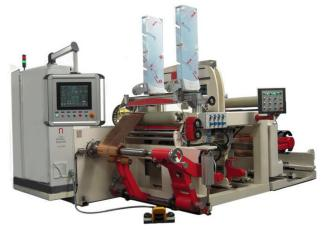
Foil winding machines are typically used for the manufacture of high current Low Voltage (LV) transformers with windings in copper or aluminum foil. They can be equipped with cold compression or tig welding devices, automatic insulation paper feeders and tape feeders; machine is fitted with expandable mandrels. The machine control and programming are made by a CNC and a user-friendly display.
